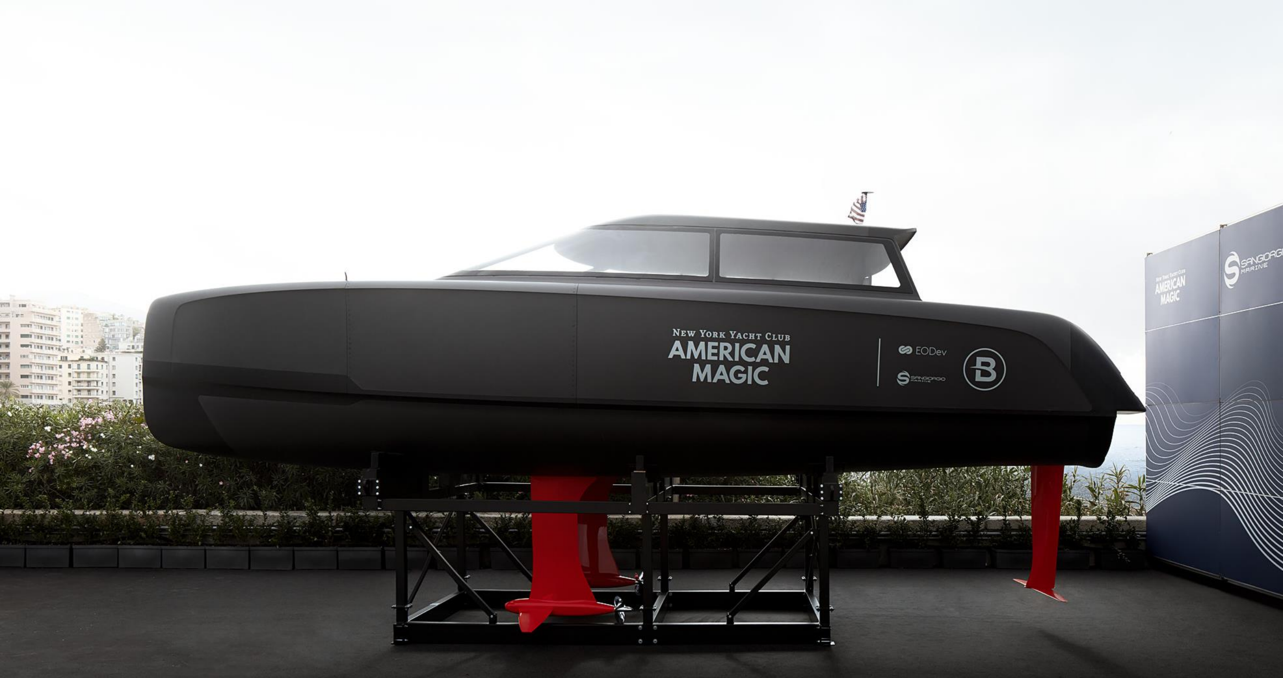
Bluegame BGH-HSV – the America's Cup chase boat with dual foil-fuel cell technology, launched in March 2024 and now undergoing sea trials
